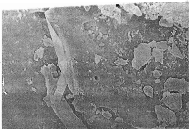
Fig. 30. SEM fractograph of tear specimen filled with 30 phr of size 4 filler.
