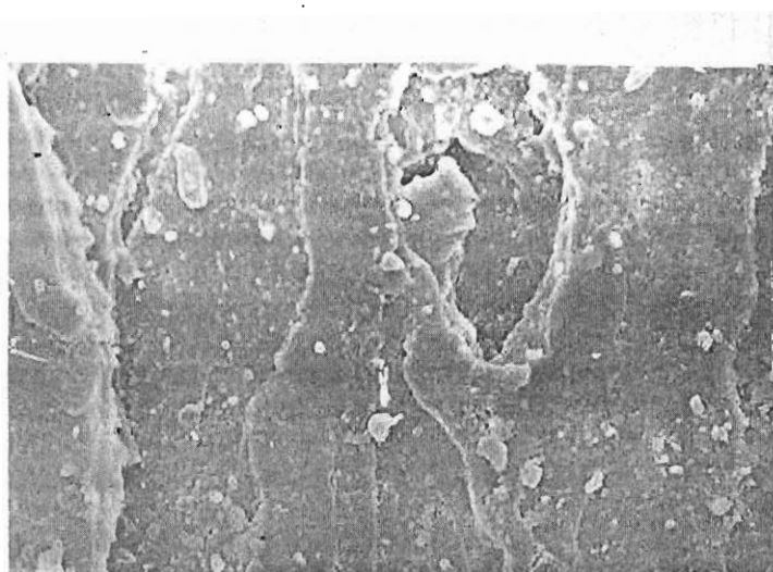
Fig. 27. SEM fractograph of tensile specimen filled with 30 phr of size 1 filler.
